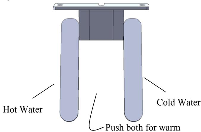
The angle of the levers can be adjusted by loosening the set screws on the hinges and re-setting them at the desired angle.
