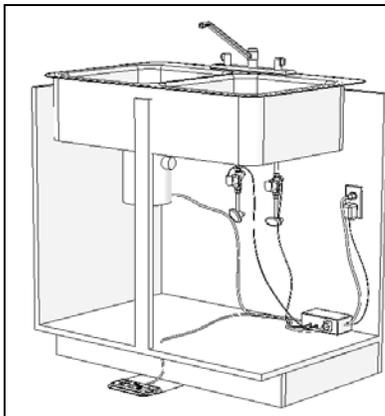
This is a picture of a typical installation of the Foot Faucet system. **TURN OFF WATER SUPPLY VALVES.** Drill a 1/4" hole in the floor of the cabinet for the control cable, then cut out a 3.25" section of each water supply tube and place the Foot Faucet valves in-line (valve must point correct direction). That's all there is to it!
