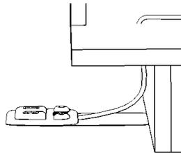
3. Cut out a 3.25" section from each water supply tube and place Foot Faucet valves in-line. Be sure valve is pointing the correct direction. The arrow on the valve should point in the direction of water flow (the end with the electrical connectors points toward the sink). If you have something other than 3/8" plastic or chromed tubing, you may have to get some adaptive fittings from your local hardware store.
