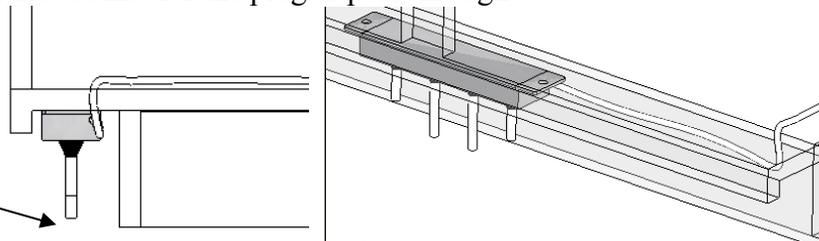
3. There are options for this. (a) Cut out a 3.25" section from each water supply tube and place Foot Faucet valves in-line. (b) Get Threaded hose with 3/8" compression end for the Foot Faucet valve and use just the threaded part of the supplied fitting. (c) Your particular arrangement may require additional hardware.
