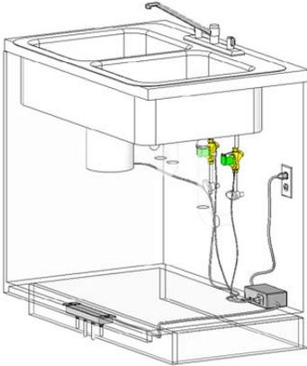
This is a picture of a typical installation of the Foot Faucet system. **TURN OFF WATER SUPPLY VALVES.** Mount pedal assembly to underside of cabinet with 1/4" (supplied) bolts, drill a 1/2" hole in the floor of the cabinet for the control cable, then cut out a 3.25" section of each water supply tube (or use a threaded hose fitting) and place the Foot Faucet valves in-line (valve must point correct direction). That's all there is to it!
